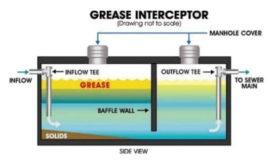
Wastewater flows from the main sewer line into the chamber on the left, where the grease floats to the top, to the left of the baffle wall. Cleaning removes the grease layer shown in the first chamber.
